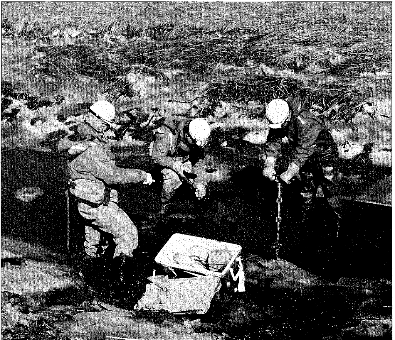
ENGINEERS ARE MONITORING LEACHATE DISTRIBUTION AT NEW YORK CITY'S FRESH KILLS LANDFILL, THE LARGEST LANDFILL IN THE WORLD. THE IT ENVIRONMENTAL DATABASE-MANAGEMENT SYSTEM WILL STORE AND MANAGE ALMOST 300 PARAMETERS FOR THIS PROJECT. PHOTO COURTESY IT CORP.
